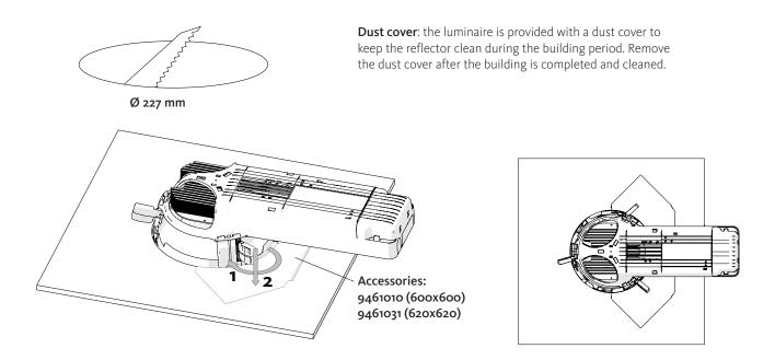
**Mounting in soft ceiling tiles**: Place the weight distribution plate straight under the luminaire housing.
