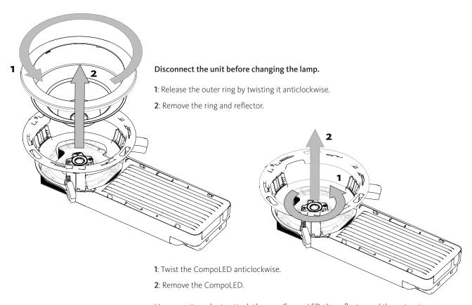
Use opposite order to attach the new CompoLED, the reflector and the outer ring.
