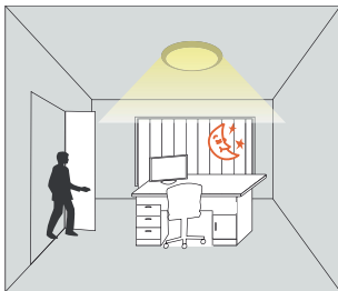
With movement, the light is triggered on by the detector.
